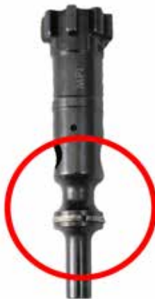
Incorrectly Staggered Gas Rings
