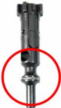
Correctly Staggered Gas Rings
